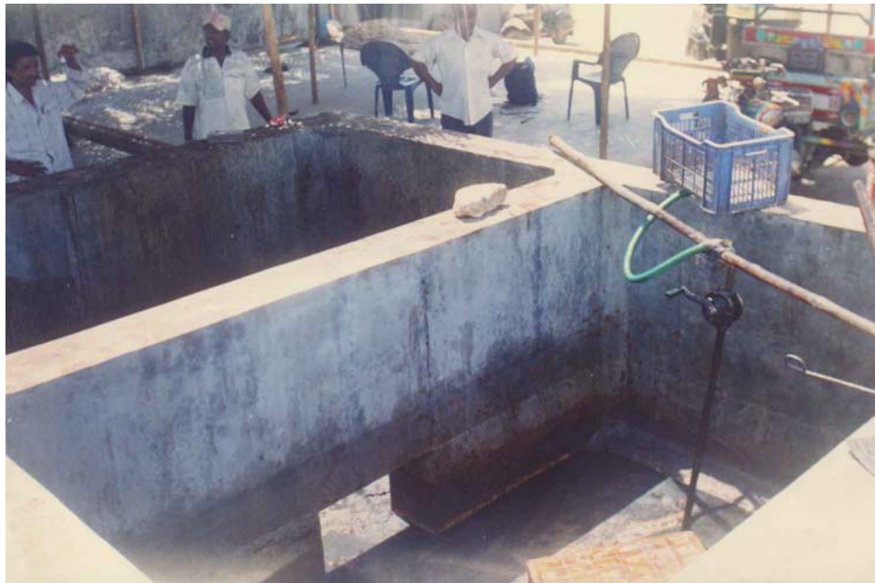
Photo 10: The twin tanks are used for producing liver oil. The pieces of liver were dumped into the tank and exposed to sunlight. No chemicals were added except a little soda. A simple hand operated pump was used to fill up the drums from these tanks after about a week (or earlier as per demand). This is an improvement over the method shown in Mike Pandey's film where the liver is shown being cut into strips and stuffed into the drums directly.
