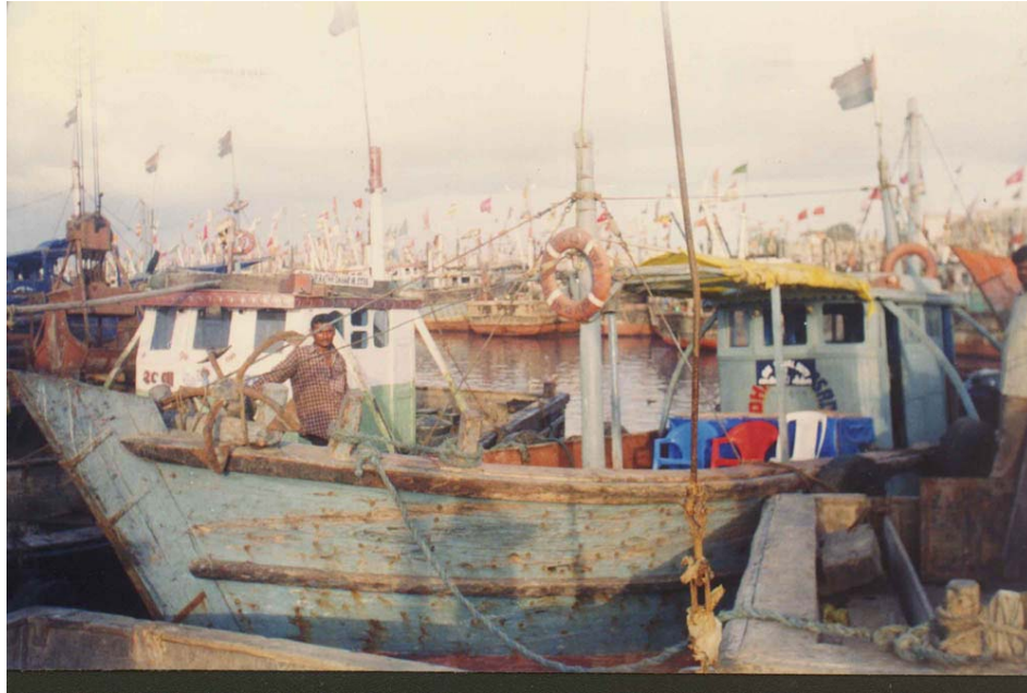
Photo 3: This fishing trawler was hired by the coast guard on a four-month contract for enforcing the fishing ban. Note the yellow polyethylene make-shift shelter and plastic chairs. It is possible to incorporate modifications such as a better shelter for larger number of chairs and ladder.
