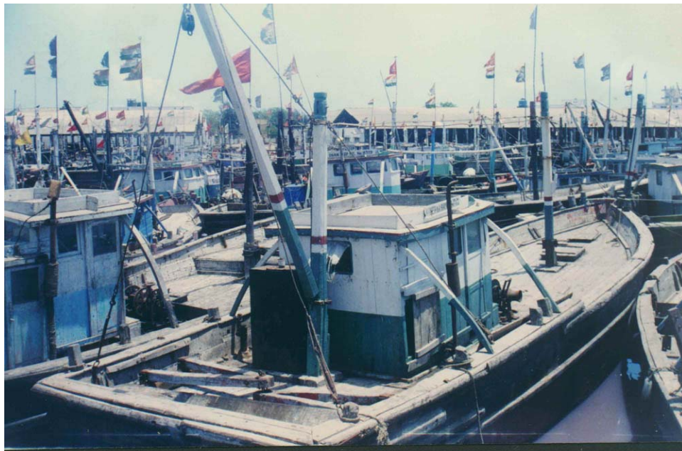
Photo 2: A typical locally-made wooden fishing trawler showing space available on the deck. Some of them are marginally longer / wider by a few feet. The hatches seen in the front are for insulated containers for ice and the fish catch.
