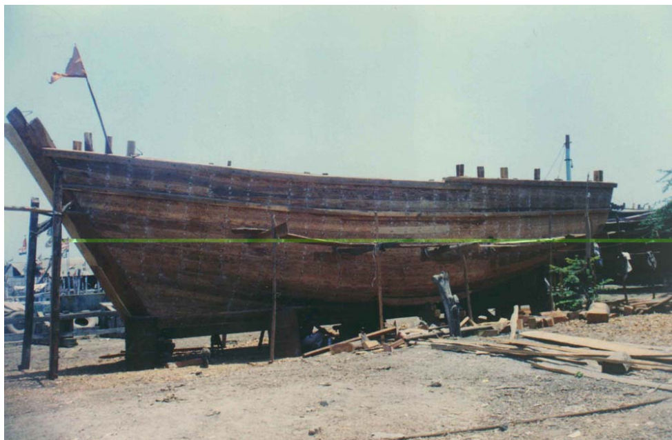
Photo 4: A wooden fishing trawler under construction at Veraval harbor by local craftsmen.
