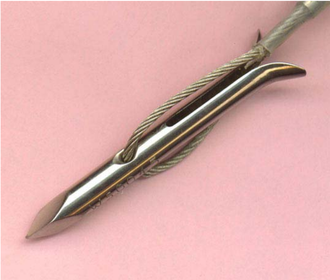
Close up of the tag anchor. It is 2" long and made of stainless steel. An identification number is engraved in the side.
